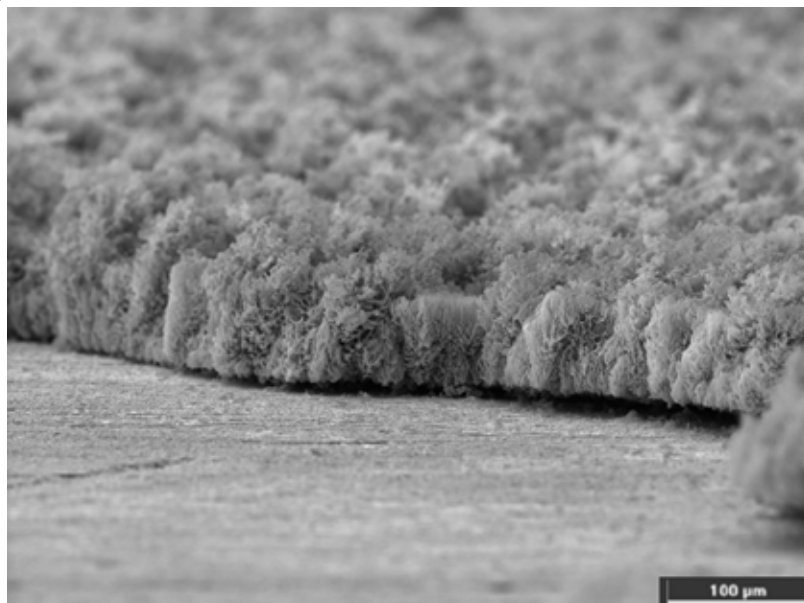
Figure 1. SEM-image of electrodeposited silicon
