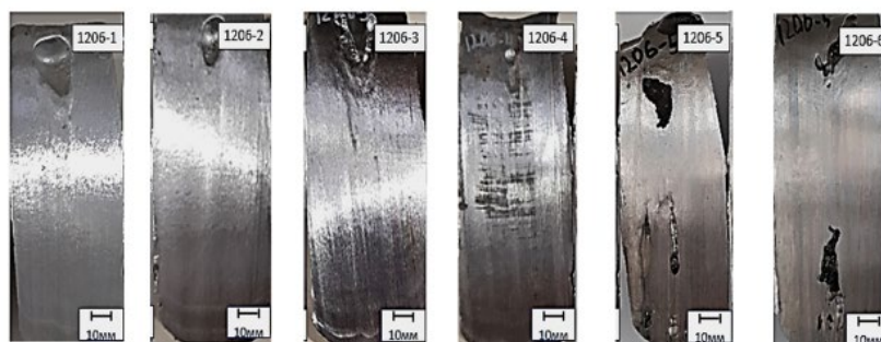
Figure 1. Templates of Fe-13Cr-(N, Mn, Mo, V, Nb) steel ingots when determining K_s
