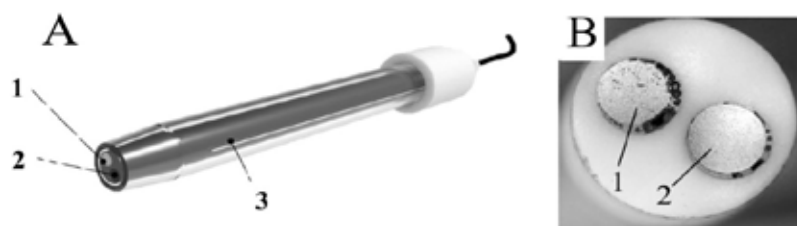
Figure 1. The «3 in 1» sensor: (A) – general view and (B) – photograph of working surface: 1 – working electrode (impregnated graphite), 2 – auxiliary electrode, 3 – reference electrode
