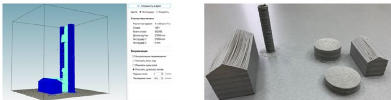
Figure 1. Cutting layers for printing (left). 3D-printed models of objects (right)
