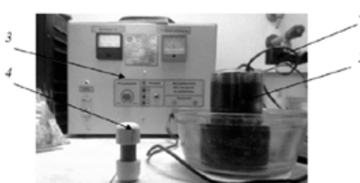
Figure 1. Assembly of the electrochemical etching stand: 1 – clamp; 2 – glass cup with steel tape; 3 – rectifier, 4 – prepared sample
