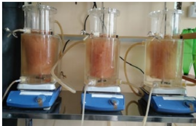
Figure 1. Automated laboratory bioreactors using the Anammox technology.
