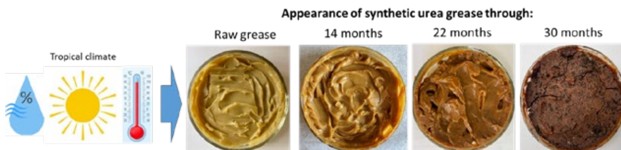
Figure. The change in the appearance of urea grease when exposed to tropical climates.
