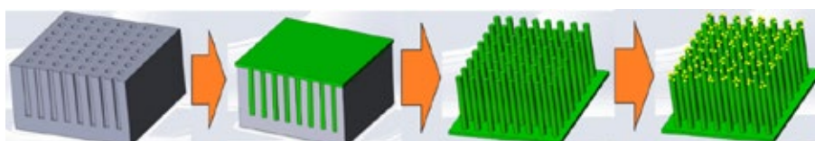
Figure 1. Schematic diagram of the production of a nickel-palladium catalyst
